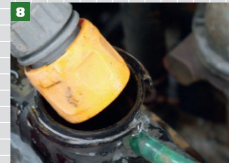
8 Now stick a hosepipe in the top and allow water to run through the radiator for five minutes or so. Once done, turn it upside down, put the hosepipe in the bottom outlet and repeat the process.
