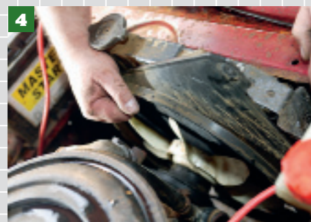
4 If fitted, unbolt the cooling fan shroud and carefully remove it. You may also need to unbolt the fan to allow enough room to withdraw the radiator.
