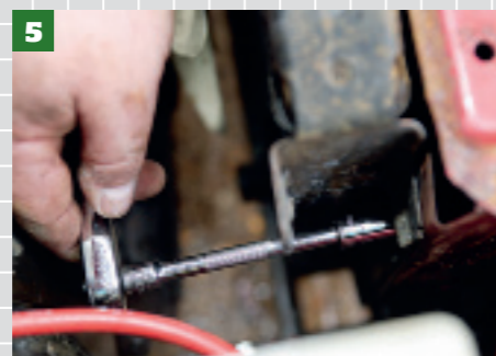
5 Then unbolt the radiator. There are usually four tapered bolts holding it to the front panel.
