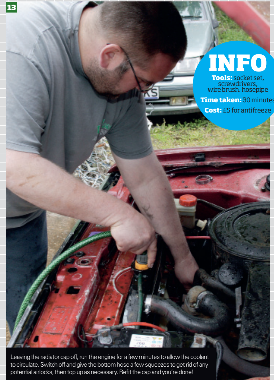
8 Now stick a hosepipe in the top and allow water to run through the radiator for five minutes or so. Once done, turn it upside down, put the hosepipe in the bottom outlet and repeat the process.
