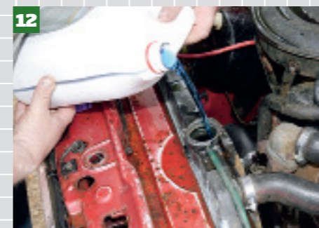
12 Now refill the system, remembering to add the correct quantity of antifreeze (usually around 15 per cent of the total coolant capacity).
