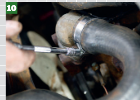
10 Along with the top and bottom hoses, replacing any worn jubilee clips with new ones where needed.
