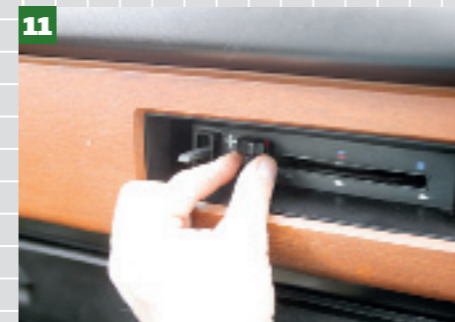
11 Slide the heater control to the hot position. This will help prevent any air locks when you refill the system.
