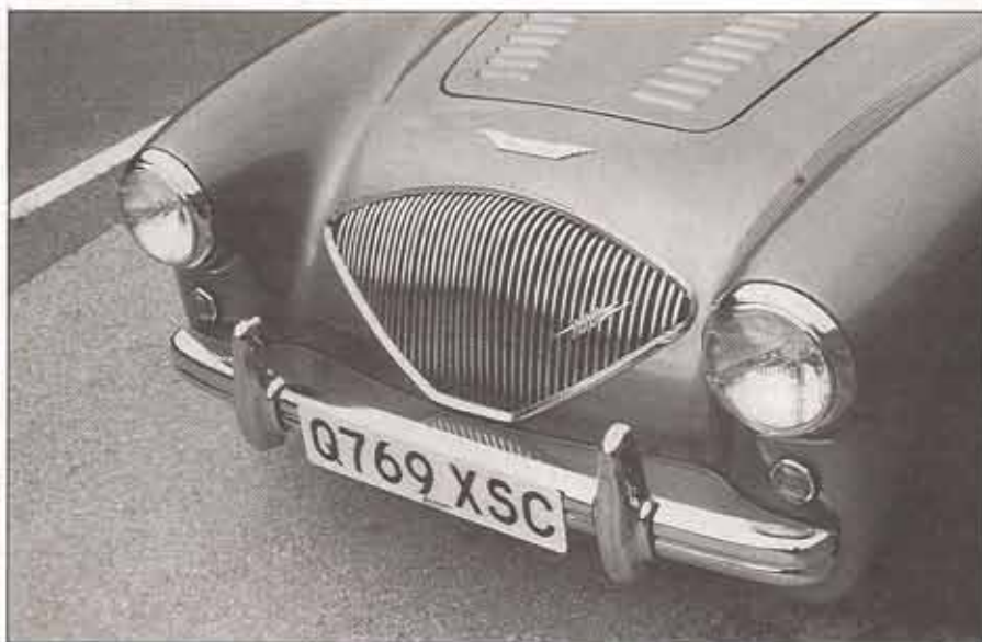
HD100 uses original equipment Healey 100/4 radiator grille, bumpers, badges, handles etc. These items are available off-the-shelf thanks to high demand from owners of rust-free original cars in Australia and USA.
