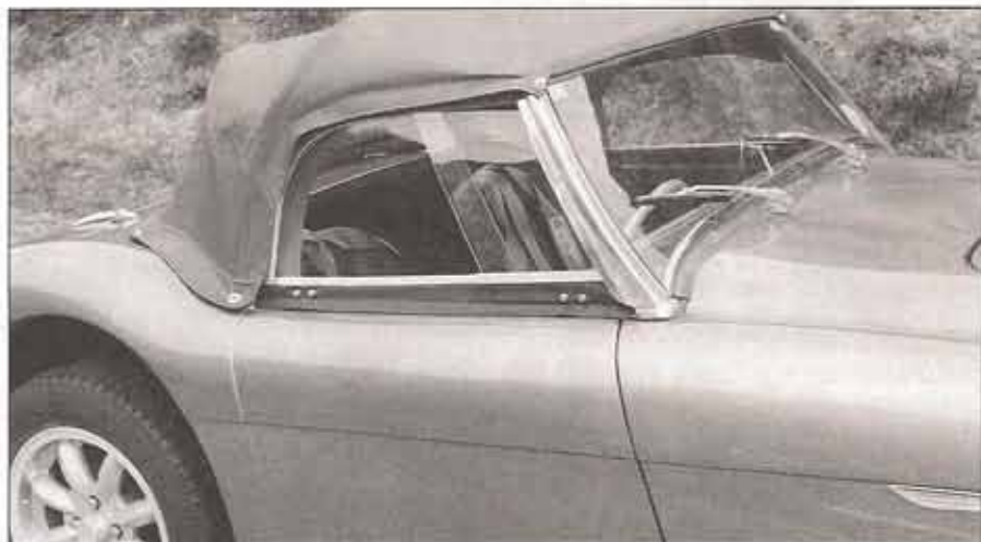
Above: Haldane makes own screen surround to fit original 100/4 glass. Below: latest HD100 chassis boasts brand new Ford Sierra 2-litre twin-cam with 5-speed gearbox. Engine is fuel injected and has full management system.
