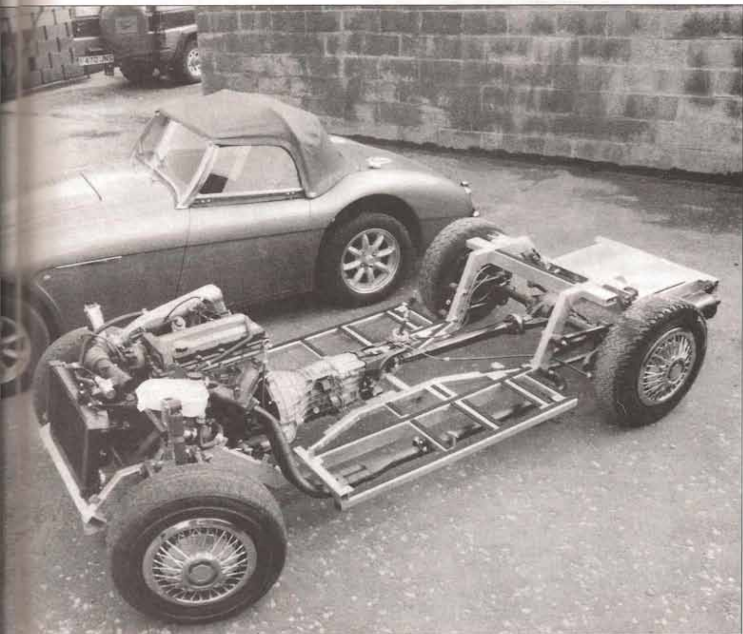
Above: Haldane makes own screen surround to fit original 100/4 glass. Below: latest HD100 chassis boasts brand new Ford Sierra 2-litre twin-cam with 5-speed gearbox. Engine is fuel injected and has full management system.
