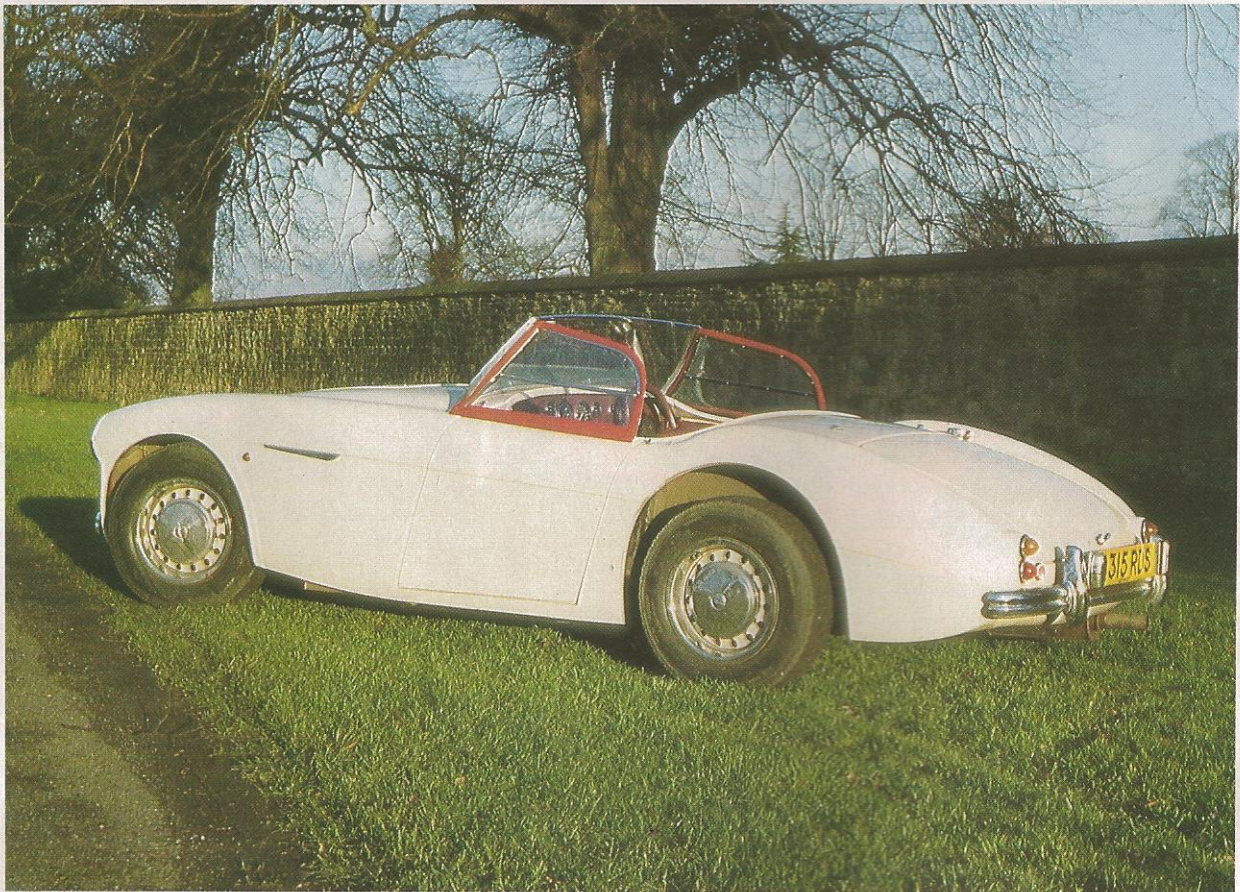
Substantial ladder-frame chassis carries high-quality semi-monocoque fibreglass bodyshell.
